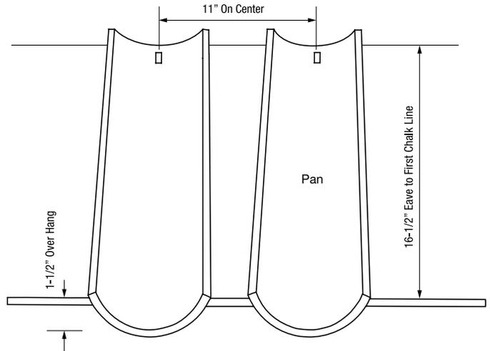
3. Install pans along eave line between birdstops by aligning the top edge of the pans with the horizontal chalk line marked at 16 1/2" for the eave.
