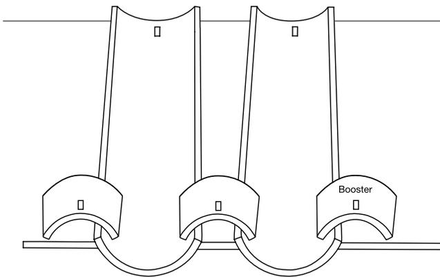
5. Cut off 3" booster piece along the factory "score" line from each booster/starter tile.
