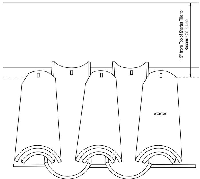
8. Make a diagonal cut at upper left corner of the starter/cover tile to match the diagonal cut of the 1-Piece "S" Tile or Claylite® field tile being used for the second course.
